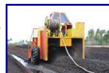
E-Compost: Conc. BMSW of 28 Brix is mixed with Press Mud
